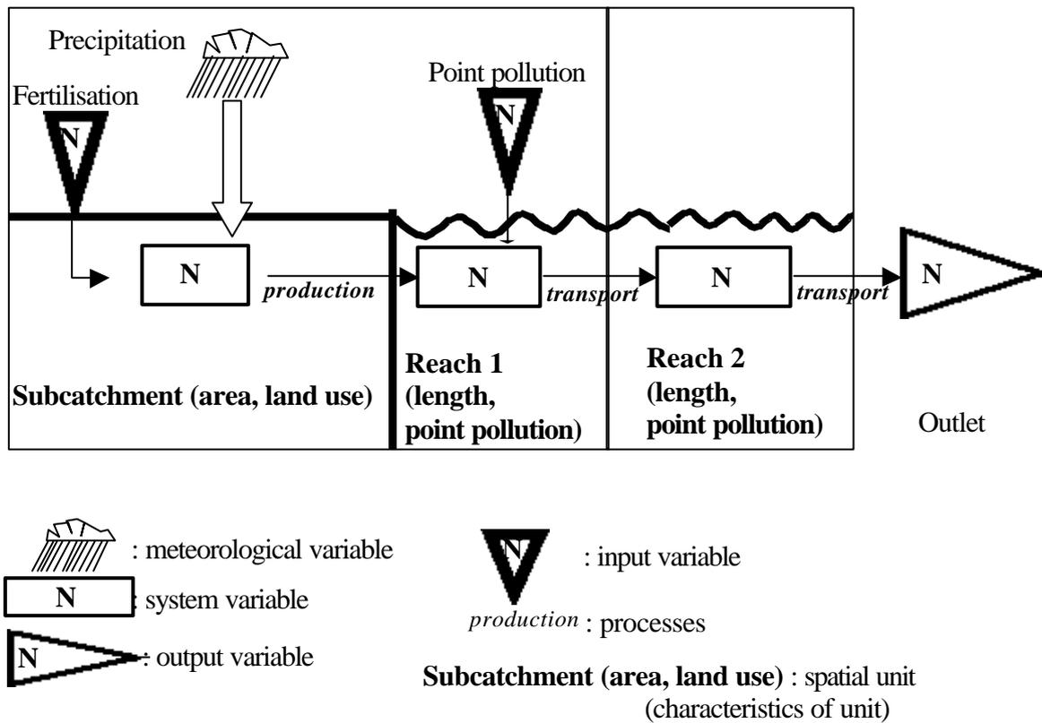
Figure 2. Schematisation of nitrogen processes in the POL model
